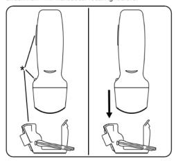
Rotate locking latch into locked position. Ensure needle guide is securely attached.
